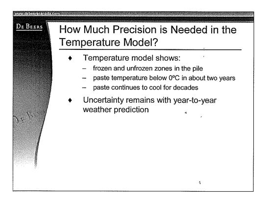
The temperature model was set up using the laboratory measured characteristics of the paste PK and the actual site weather data. The model was calibrated to the actual temperatures measured in boreholes located at the North Pile and this calibration showed that the model gave reasonable results for the conditions we see at the site now. We then ran the model with what we thought would be the most likely conditions during operation and post-closure.
