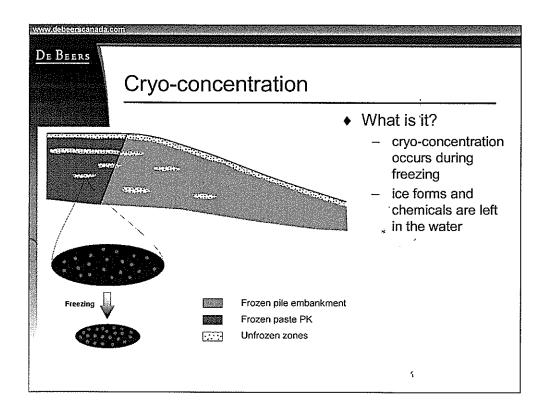
Now I'll move into the second of the three concerns relating to the North Pile, which is cryo-concentration. It can also be called freezing concentration, and occurs during freezing. As ice forms, materials in the water are expelled from the ice and remain in the water.
