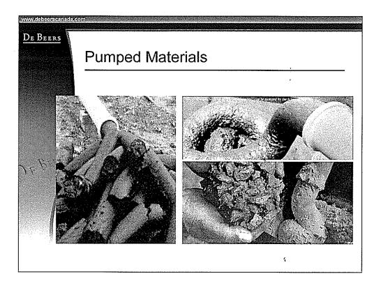
Paste is not a specific material. It is the consistency of a material with a low water content. Typical pastes are shown in the right photographs. The photograph on the left shows a drier material, what we would call a cake, that has been pumped. A slurry would be much wetter than the materials shown in these photos. In many applications, pastes will be moved by pumping through pipelines.
