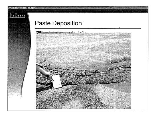
This photograph shows how paste tailings flow. You can see that at the leading edge there is no water being released. Compare this to what you have seen at mines using "conventional" slurry disposal methods and you see how this system reduces the amount of water that must be handled and contained.
