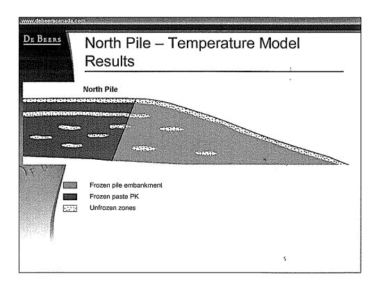
The temperature model shows that there will be frozen and unfrozen zones in the pile since the pile freezes very slowly. We are not certain about the exact distribution of the unfrozen areas in the pile, because this will depend on both the exact pattern of PK placement and the weather at the time of placement, but the operating methods are designed to accommodate this condition.
