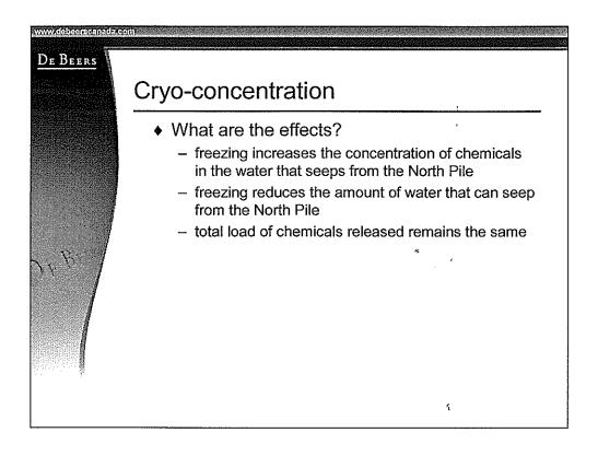
Cryo-concentration is important because it will lead to a higher dissolved solids concentration in the water that comes from the paste in the North Pile. We must also remember that the freezing process will reduce the amount of water that can come from the North Pile since more water will remain in the North Pile as ice. The result will be a smaller amount of water with a higher concentration of dissolved solids, but the total load of the dissolved solids will be about the same.
