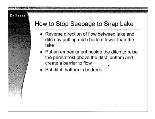
The issue was that water would seep from the ditch into the lake. To resolve the issue, we have reversed the direction of that flow so that it is now from the lake to the ditch. This was done by putting the bottom of the ditch slightly lower than the lake level along as much of the ditch as possible. This also means that the ditch bottom will be in granite bedrock.
