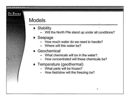
For most projects, we model or analyze for stability, seepage and geochemical performance. At cold climate or Arctic projects, where freezing is important, we also do temperature modelling, called geothermal modelling, to determine what will freeze and how fast or slow this freezing will occur.
