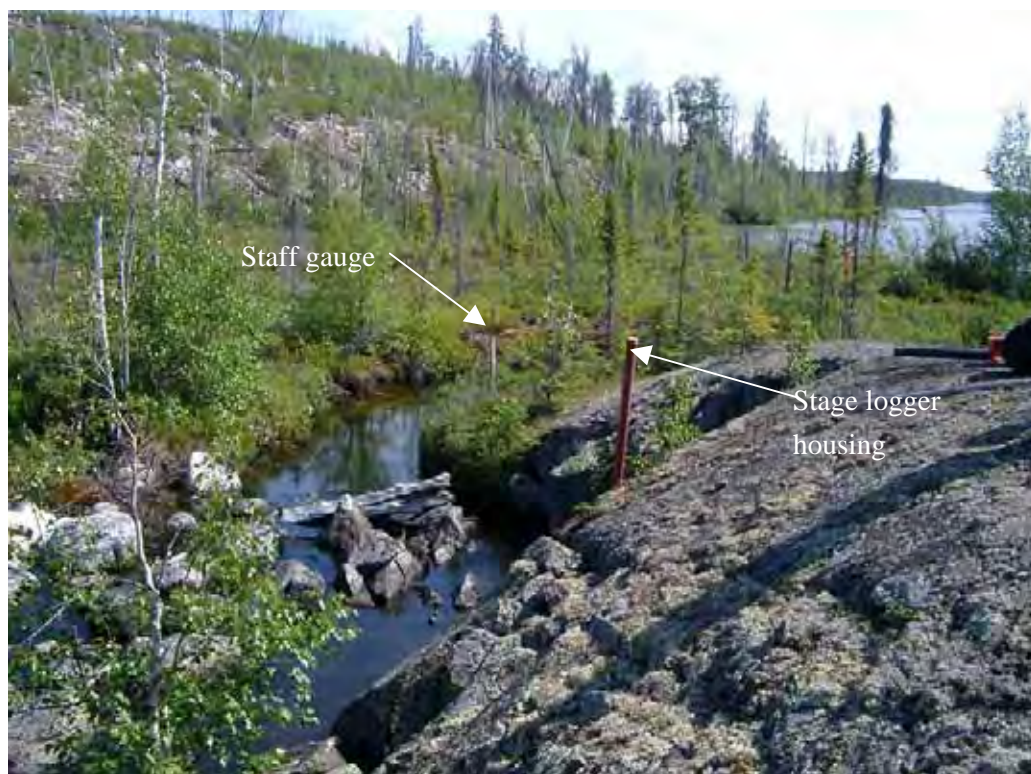
Site#6: Pressure transducer and data logger
