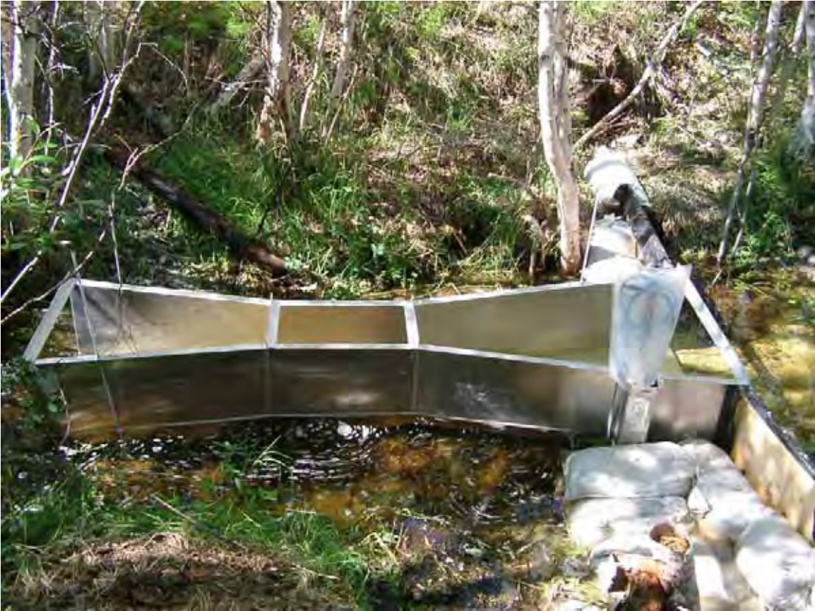
Site #1: Hydrometric gauging station with installed Parshall flume
