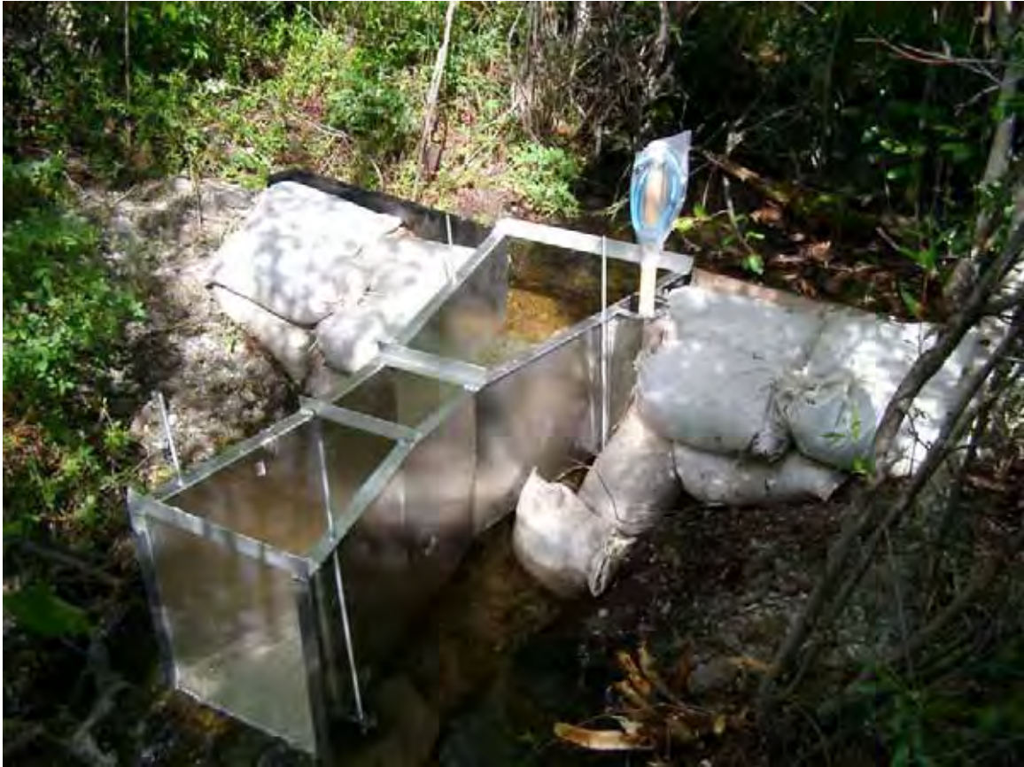
Site#3: Hydrometric gauging station with installed Parshall flume
