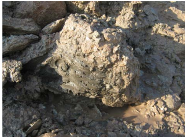
Photo 13: Tailings/PAG mine rock interface, no mixing (co-mingling) has occurred
