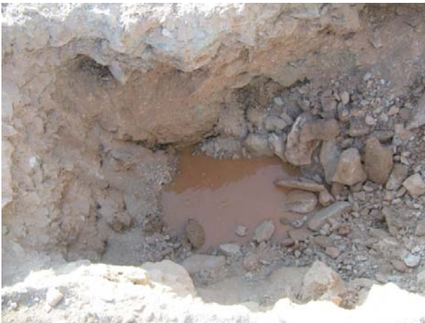
Photo 12: Standing water test pit excavated through PAG mine rock pad in Photo 3
