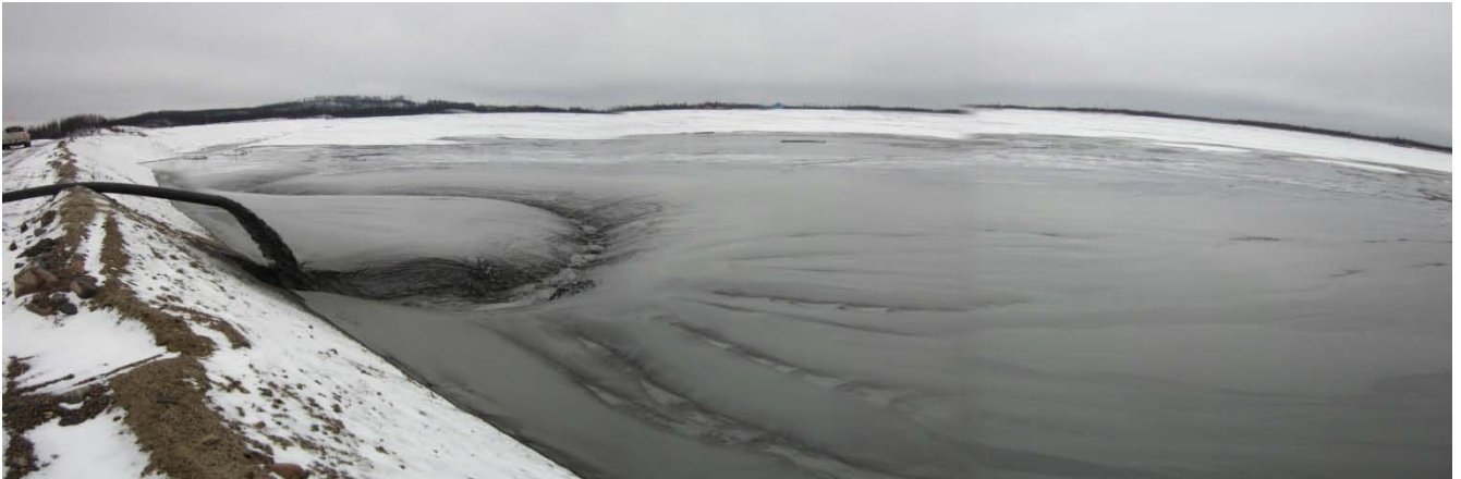
Photo 29: Musselwhite Thickened Tailings Deposition
