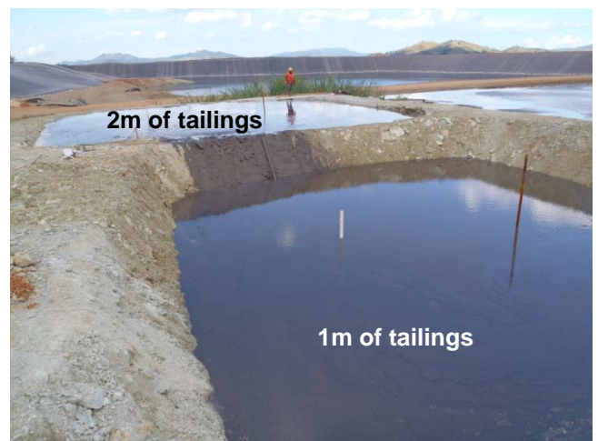
Photo 22: Deposition test cells after initial filling
