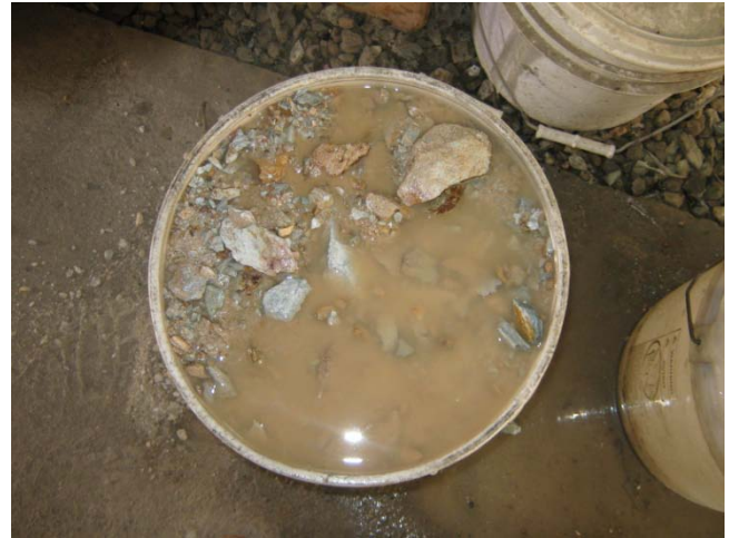
Photo 9: Measuring void ratio of PAG mine rock
