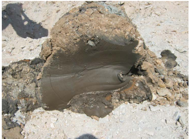
Photo 17: Tailings/PAG mine rock interface, no mixing (co-mingling) has occurred.
