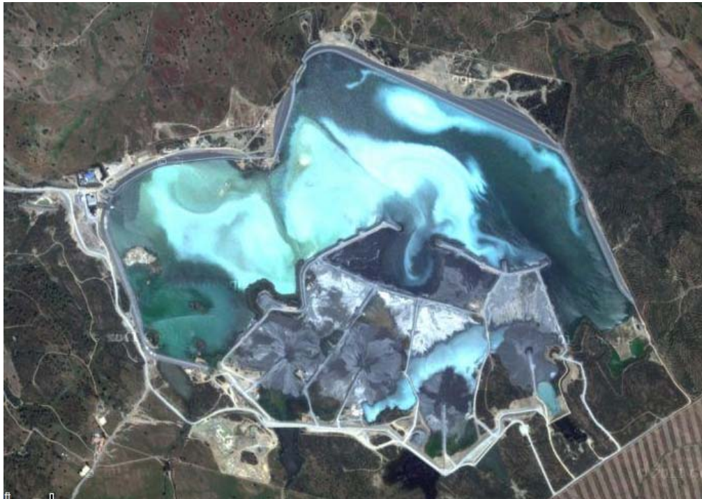
Photo 3: Paste Disposal at the Initial Four Cells at Neves Corvo
