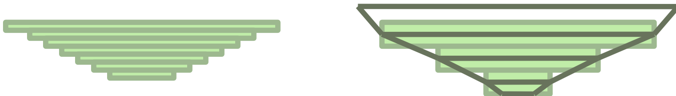
Figure 37. Various solutions to fitting a cross-section –trapezoidal layers compared to multiple rectangular layers.
