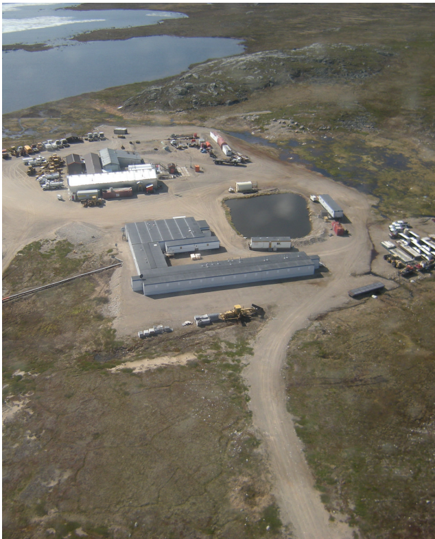
figure 23. A large stationary camp with a sewage lagoon for wastewater treatment.
