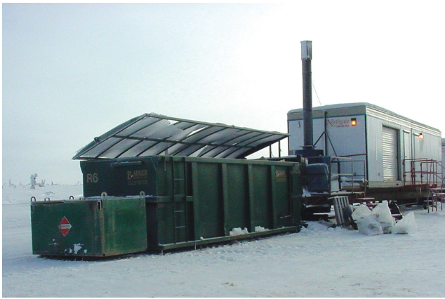
figure 20. A fuel-fired incinerator with a bin nearby to store non-combustible wastes.
