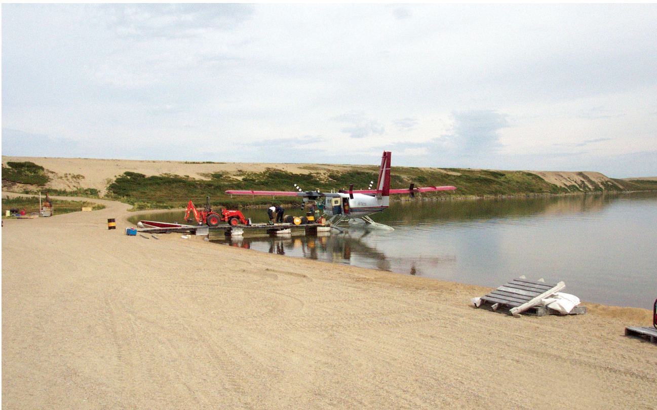
figure 12. A dock should be located in a sheltered area with a gentle shore and adequate water depth for float planes and boats.
