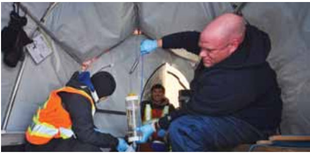
TECHNICIANS FROM GOLDER ASSOCIATES WORK INSIDE A TENT SET UP ON THE ICE OF KENNADY LAKE TO COLLECT A WATER SAMPLE THROUGH THE ICE, IN APRIL 2011.
