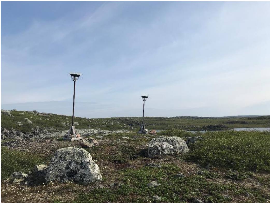
FIGURE 7. DUSTFALL STATION WITH TWO PARALLEL COLLECTORS, JULY 2019
