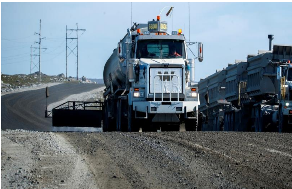
FIGURE 5. ENVIROKLEEN BULK FLUID TRUCK WITH 25 FT SPRAYER USED FOR APPLICATIONS, 2017 TO 2019
