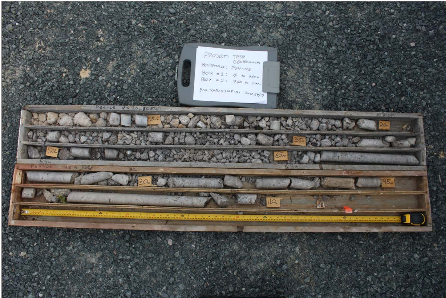
Description: Borehole P69-05, 0 m to 11.00m, Dry
