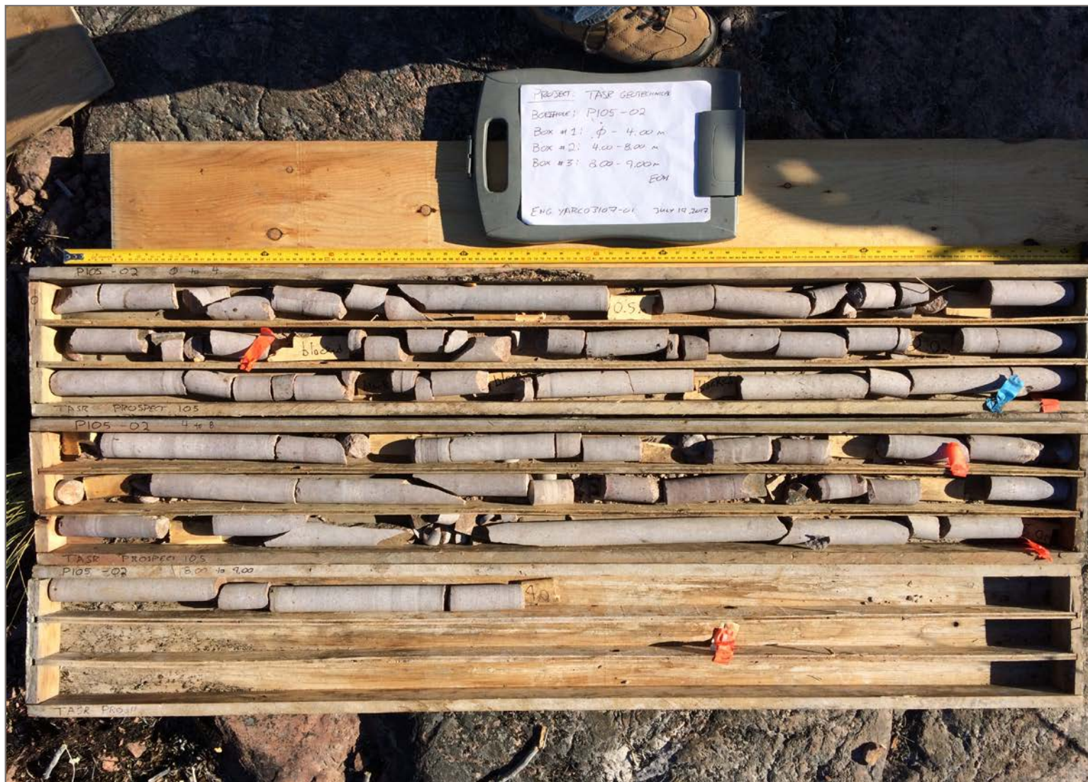
Description: Borehole P105-02, 0 m to 9.00m, Dry
