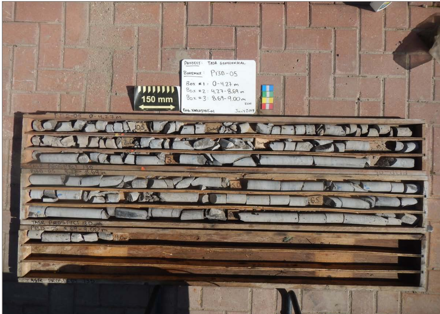
Description: Borehole P13D-05, 0 m to 9.00m, Dry
