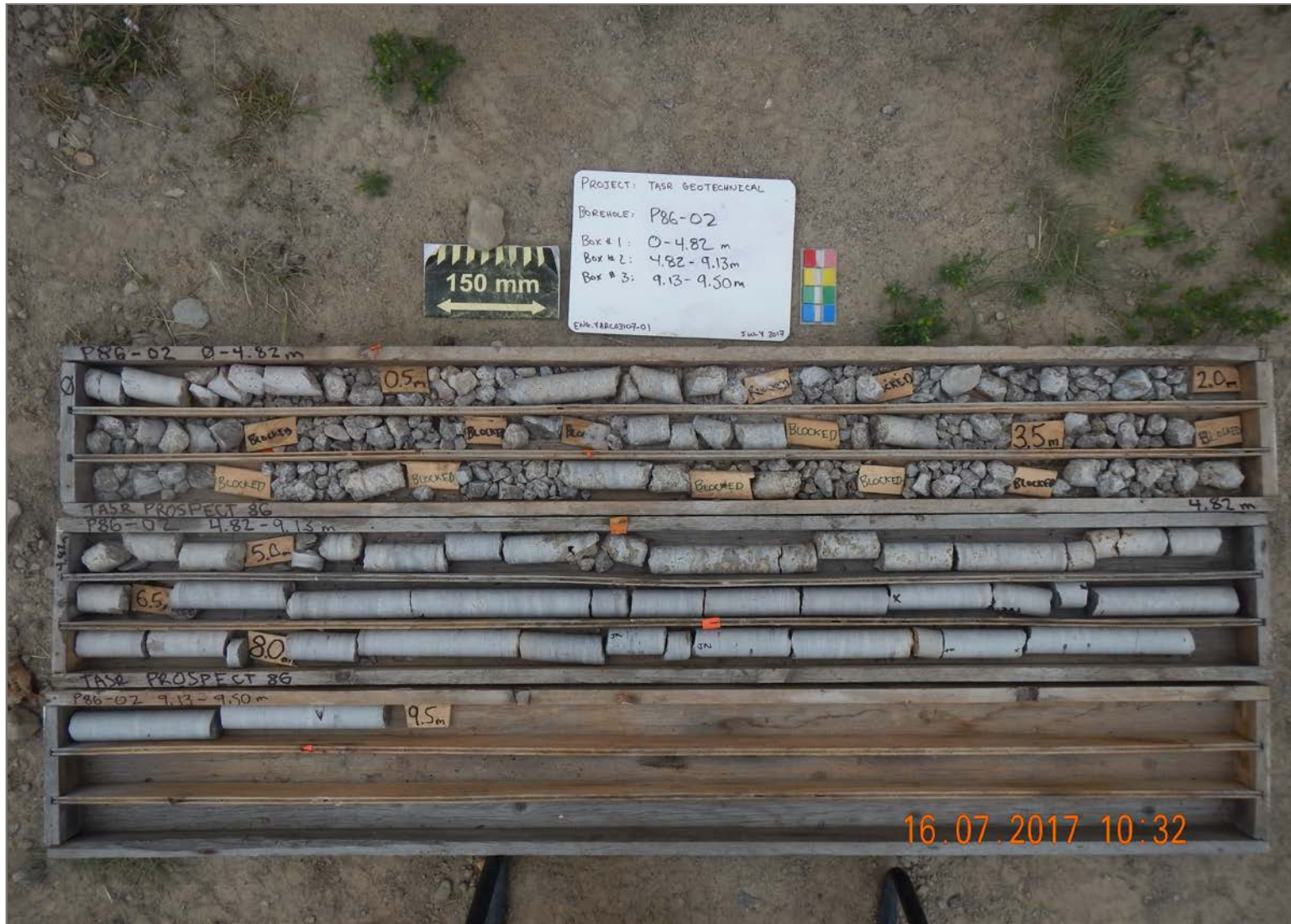
Description: Borehole P86-02, 0 m to 9.50m, Dry
