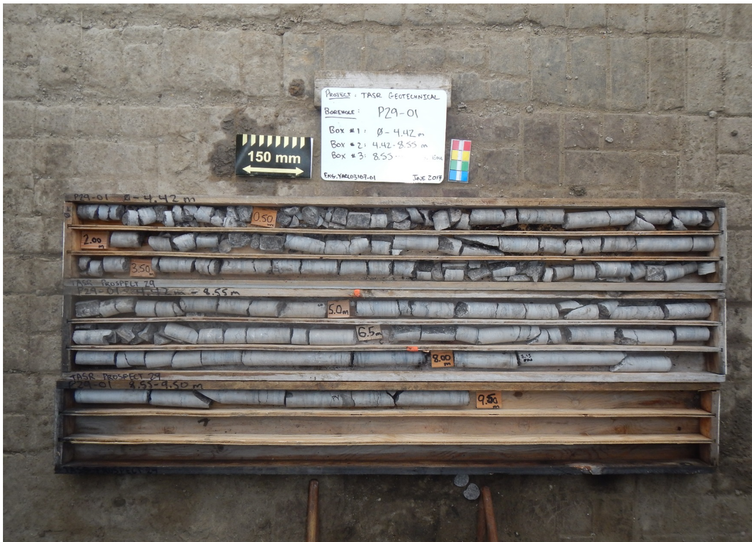
Description: Borehole P29-01, 0 m to 9.50m, Dry
