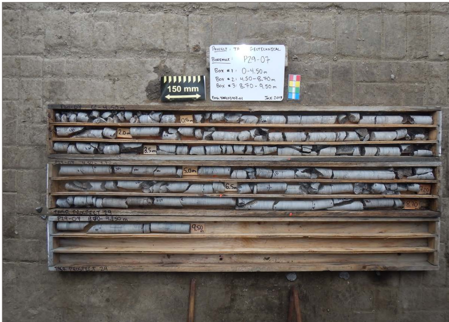
Description: Borehole P29-07, 0 m to 9.50m, Dry
