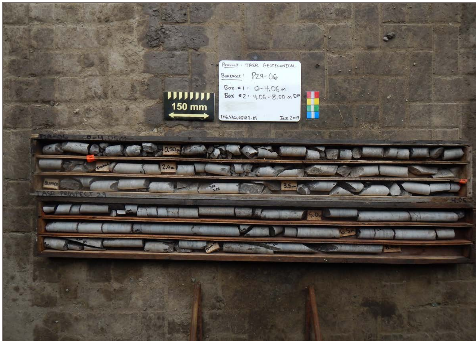
Description: Borehole P29-06, 0 m to 8.00m, Dry
