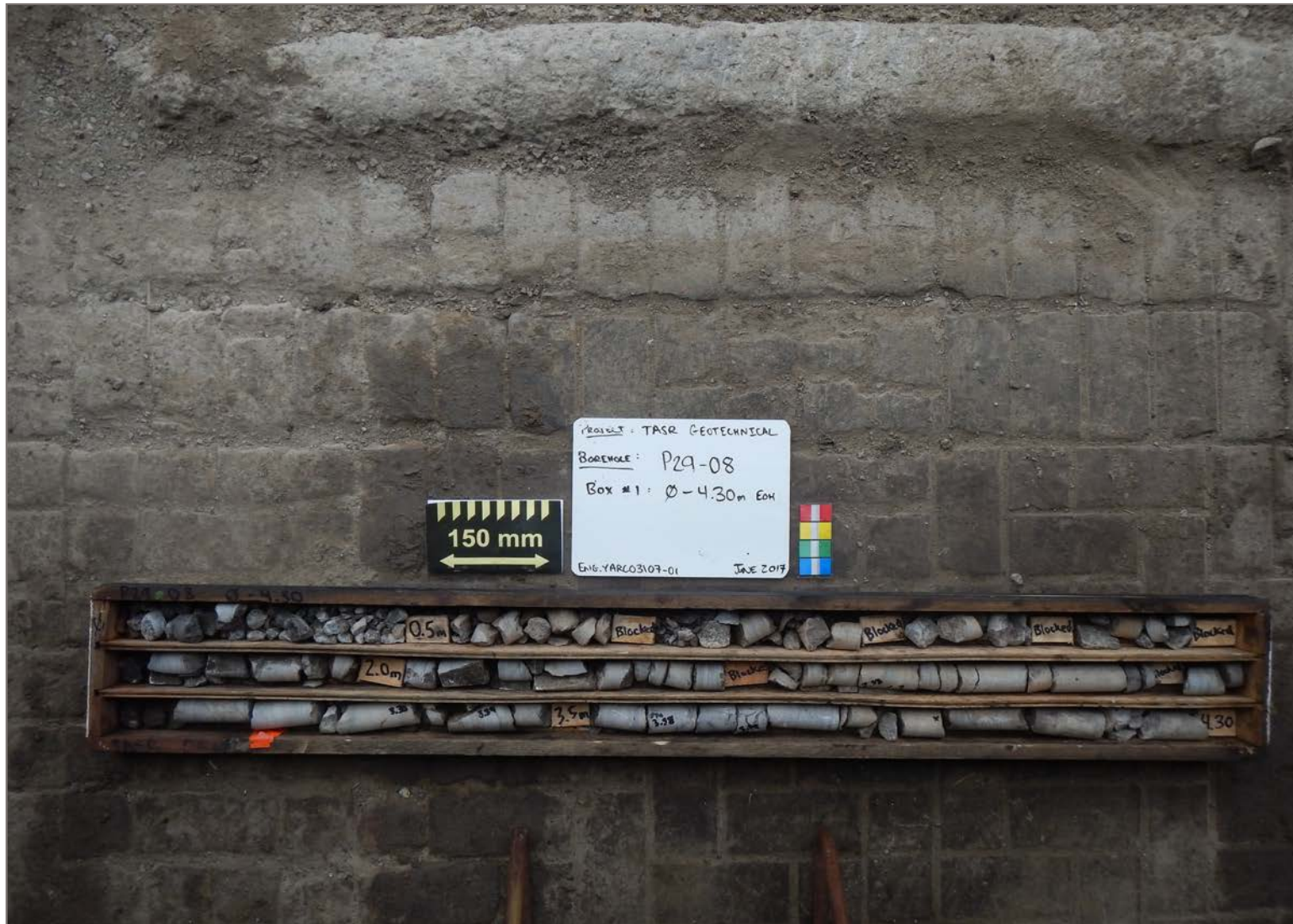
Description: Borehole P29-08, 0 m to 4.30m, Dry
