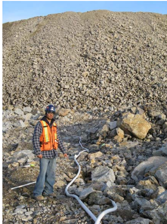
Figure 2-27. Horizontal instrument installation in full-scale Type III dump.
