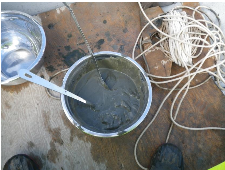
Figure 11: North Inlet reconnaissance: grab at transect location 5. Grab collected at east end of North Inlet near Station NI-5. Grey sediments (silt and clay) with thin brown surface layer; sediments more consolidated than at transect locations 1 to 4, with less moisture. Lower grab penetration. UTM coordinates (UTM Zone 12): 535063 easting, 7153300 northing.
