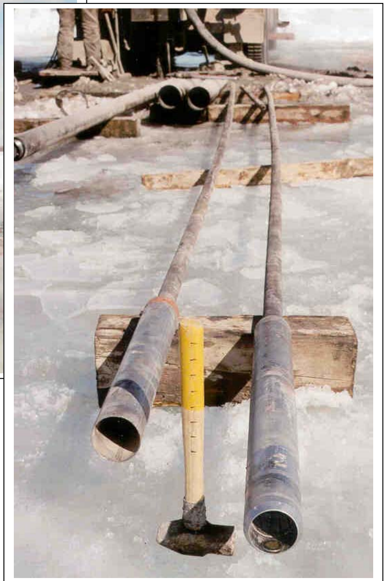
Photo 6: April 17, 2003 - Shelby Tube on left and LPT Split Spoon on right
