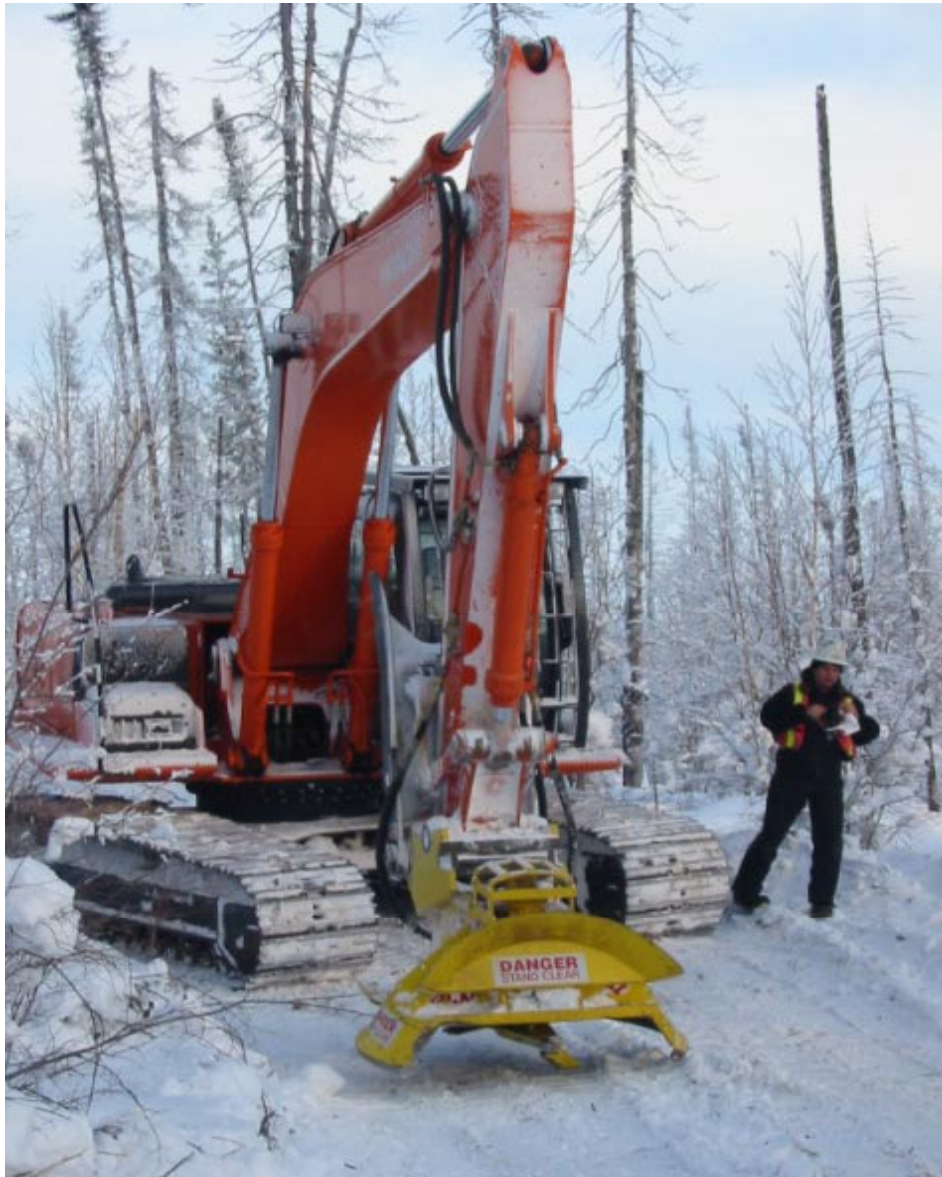
Operations: Hitachi tracked hoe with hydraulic mounted brush cutter Sahtu K'ahsho Got'ine 2004
