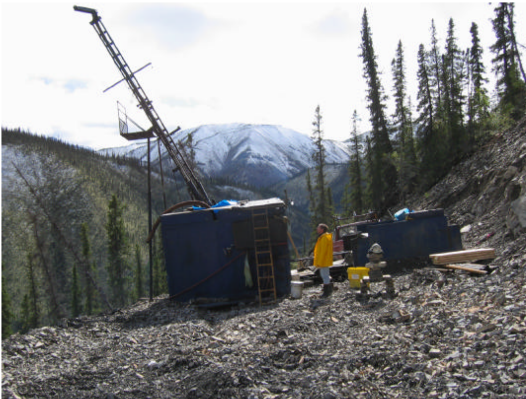
Plate 2: CZN's Long Year super 38 drill rig.
