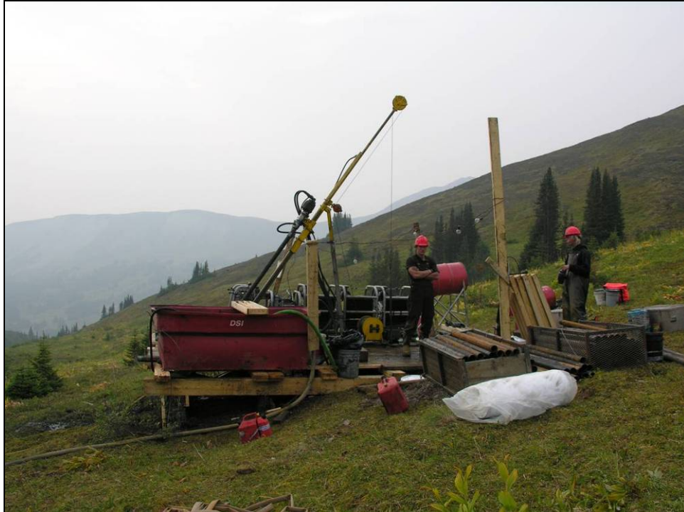
Photo 4 – Helicopter supported drilling operation
