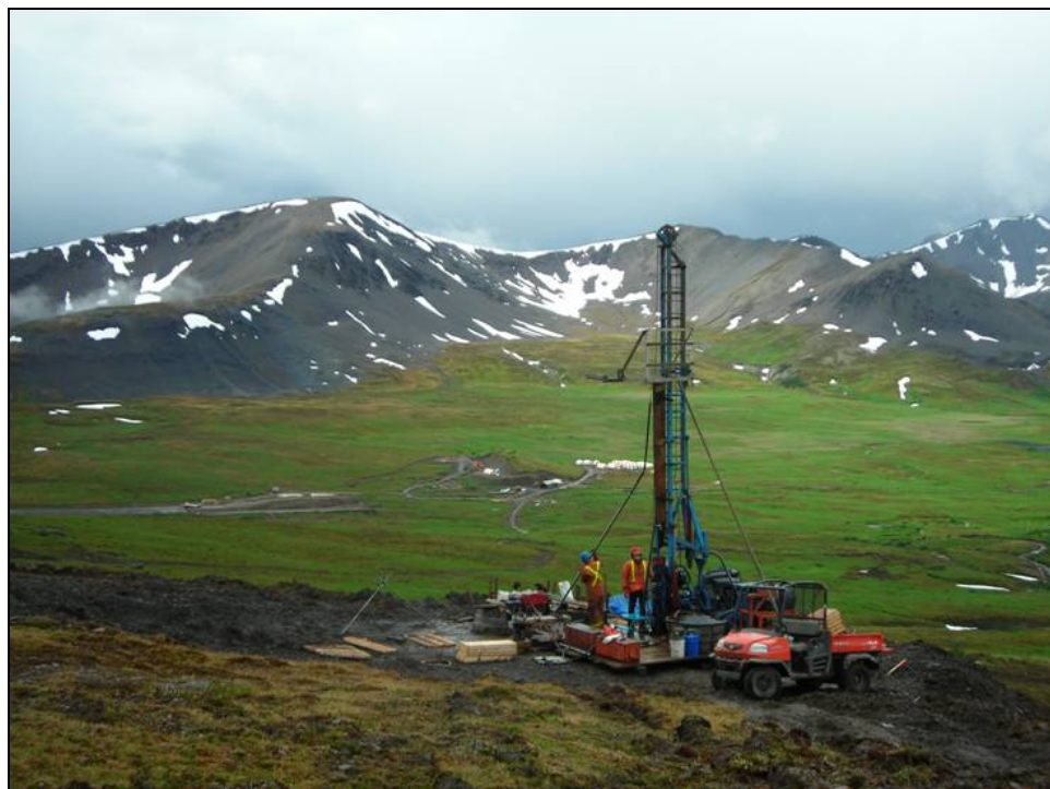
Photo 5 – Ground supported drilling operation
