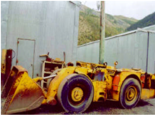
Underground Scoop Tram
