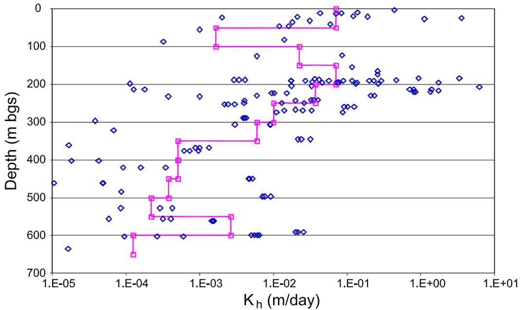
b) Measured Vertical Hydraulic Conductivity vs. Depth
