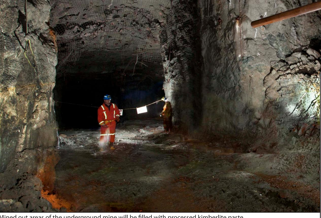
Mined out areas of the underground mine will be filled with processed kimberlite paste.
