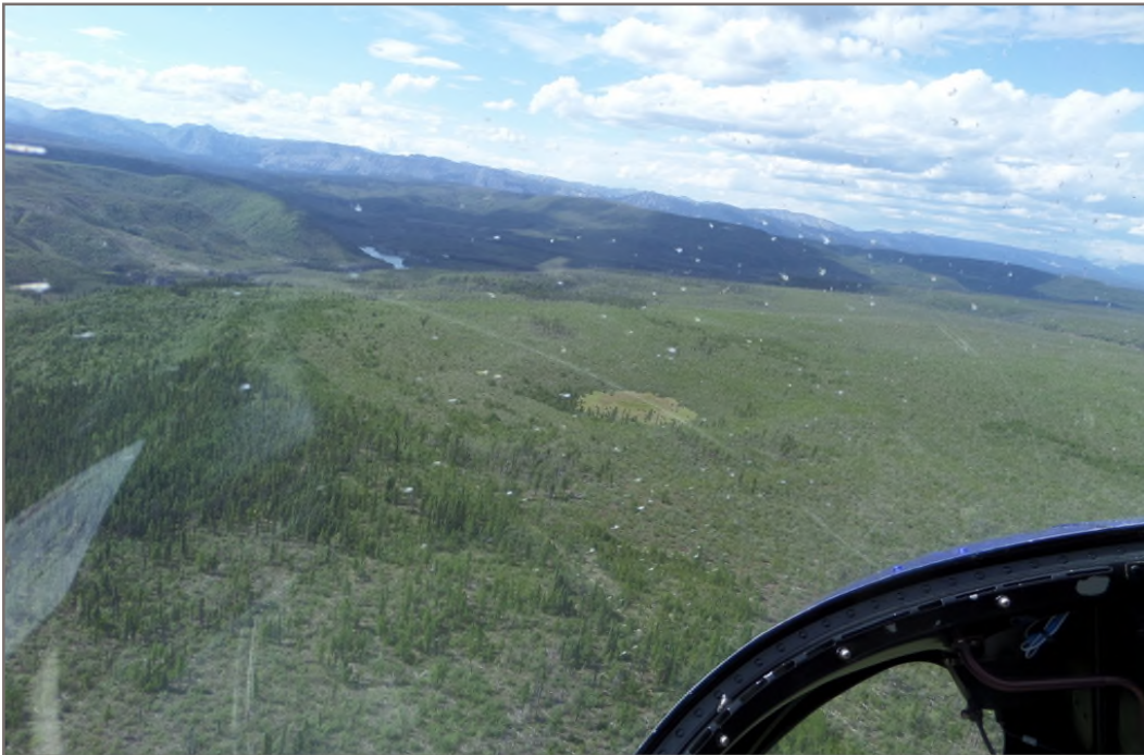
Photo 8: Looking west-northwest from about KP059.3, note lighter-coloured depression north of KP058.9. Possible sinkhole due to large size (70 m) and mapped so by Golder (2010). May be more likely a kettle (Tetra Tech EBA, 2015c). (Photo credit: Allnorth.)
