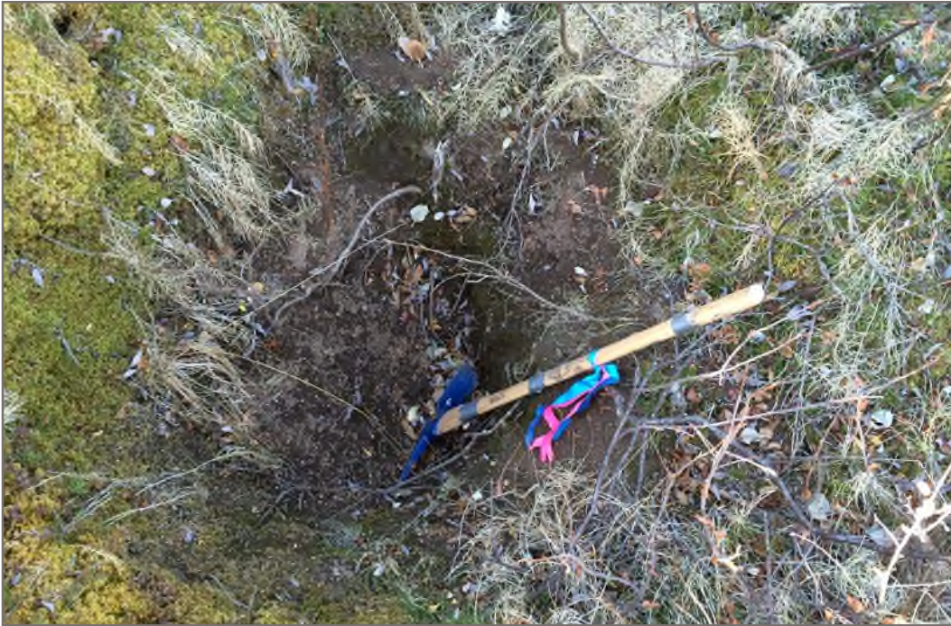
Photo 1: Suspected suffosion feature at about KP025.6. This is the largest of three micro-features in this area of the route, at about 0.6 m depth and 1.5 m diameter. This feature is nearly perfectly conical. Other features just below the route are less regular.
