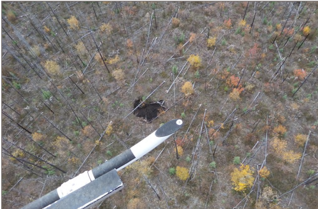
Photo 6: Suspected suffusion feature located about 70 m south-southeast of route near KP056, and estimated at about 3 m in diameter. This feature could also be thermo-karst-related. See also Photos 5 and 6 for location. (Photo credit: Allnorth.)
