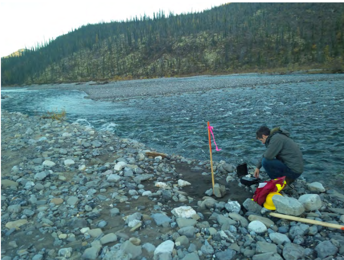
Kerry Cupit measuring turbidity at the upstream Prairie Creek station
