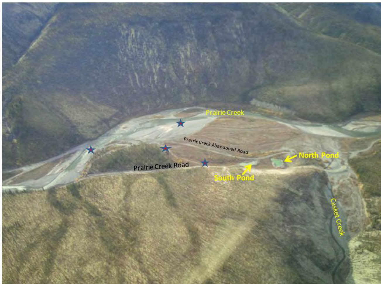
September 14, 2013: Aerial photo of Fish Compensation area after construction of ponds. The locations noted by stars are the turbidity monitoring sites.
