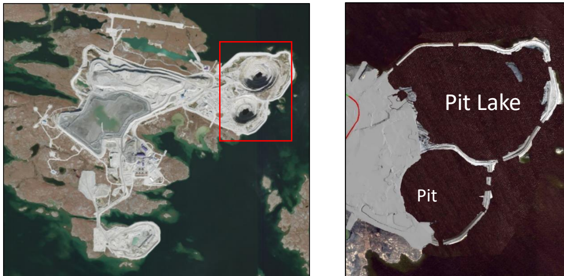
Figure 6: Diavik’s closure plan is to fill the pits with water to create pit lakes
