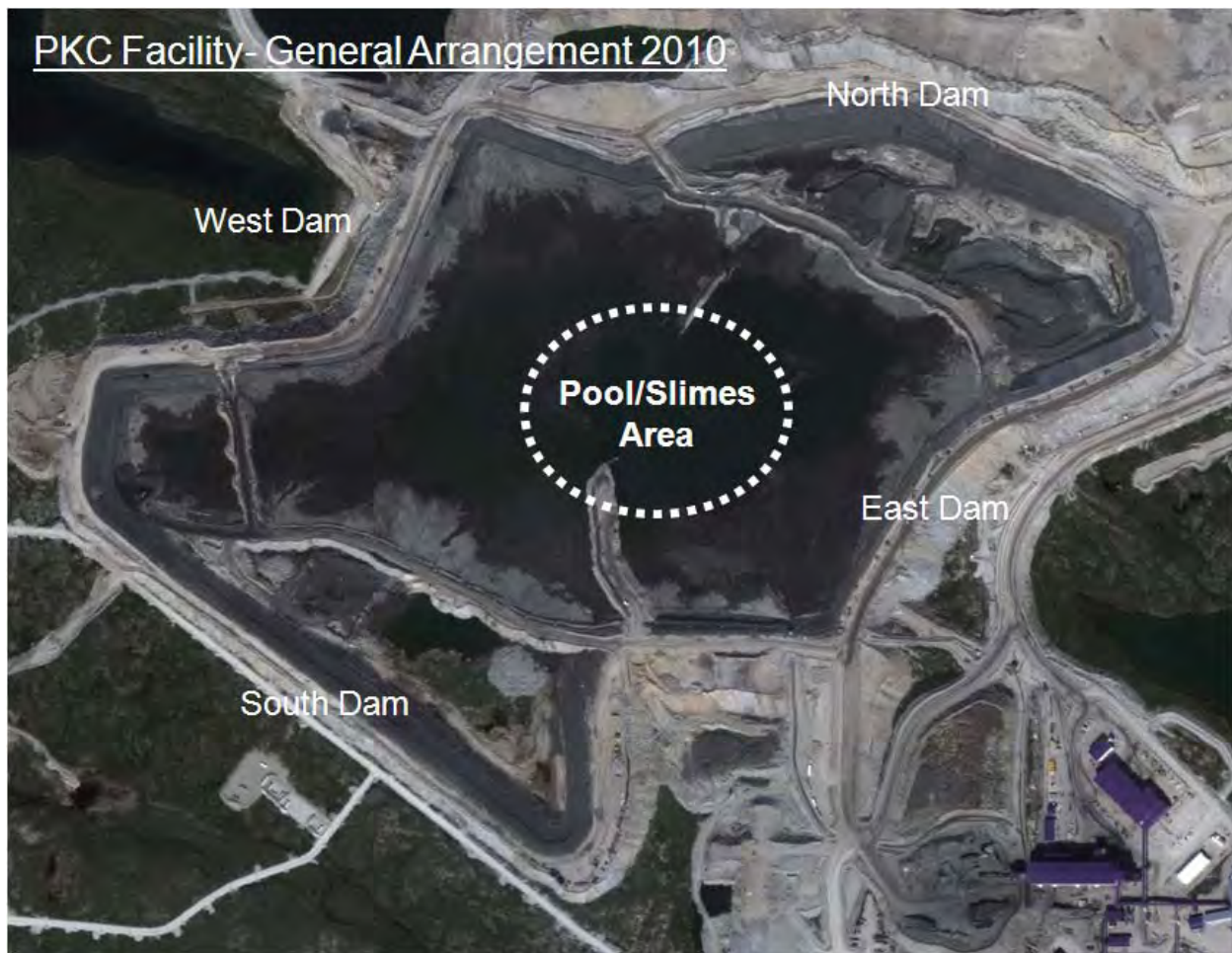
Figure 2.1: PKC Facility General Arrangement
