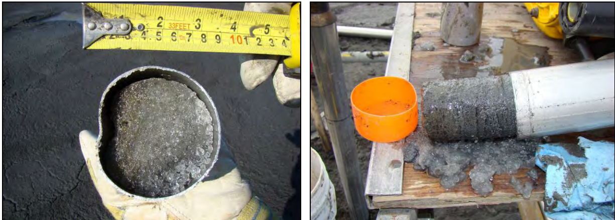
Figure 3: Core Photos from PKC2 and PKC3 Facility. Photo on the left shows ice in the bottom of a 3-inch diameter core sample collected from PKC3. On the left, photo shows frozen 2-inch diameter core collected from PKC2.
