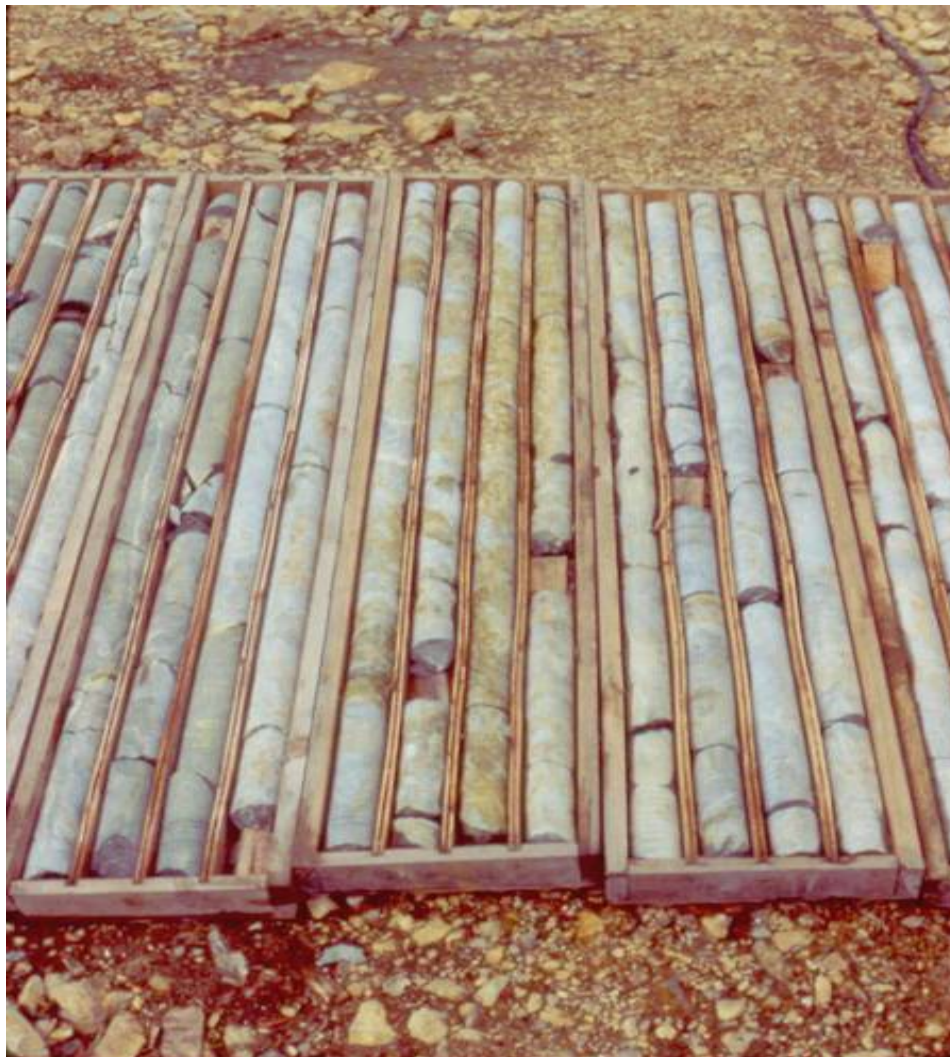
Figure 17.1 Visual descriptions of drill core provide valuable mineralogical information.
