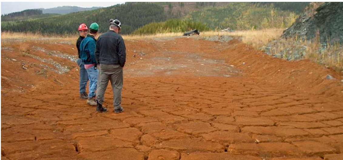
Figure 7.4 High density lime treatment sludge stored on a gravel pad to maintain aerated conditions.
