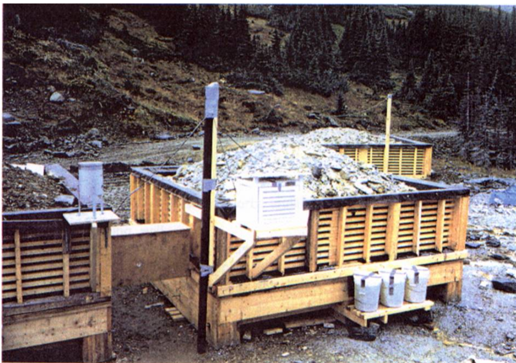
Figure 19.6 Field test pads built in a lined wooden box.
