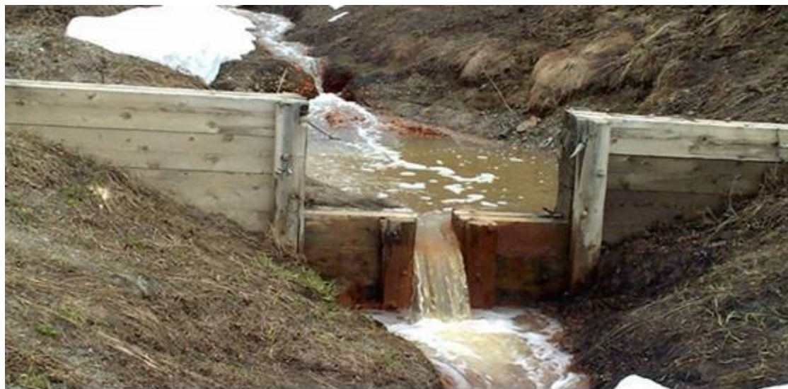
Figure 9.6 Monitoring of the rate and volume of flow are needed to calculate contaminant loadings.
